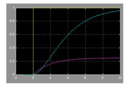
Note the difference in the shape of the curves for tank1 (pink line) and tank 2 (blue line) for the step input (yellow line). In addition, for tank 2,  $dH_2/dt$  is 0.
