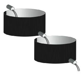
In examining the above figure, it is important to note that the water can only flow from the upper tank to the lower tank. It can not flow in the opposite direction. Thus, the tanks are said to be *noniteracting*.
