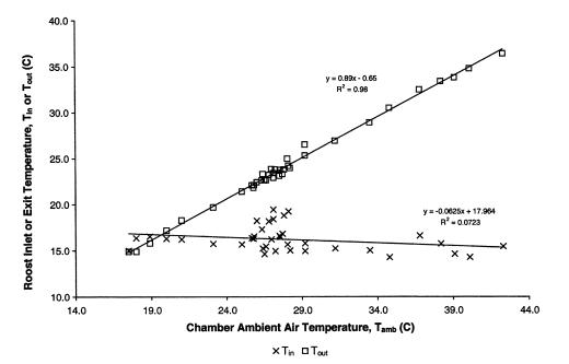
Figure 2. Roost calibration curve used to estimate roost exit temperature without birds (Tout).
