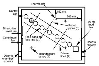
Figure 1. Chamber layout showing lighting, ventilation, roost, feeding, and watering systems in a chamber used in the studies. Light bulbs were located 1.5 m from the nearest wall.
