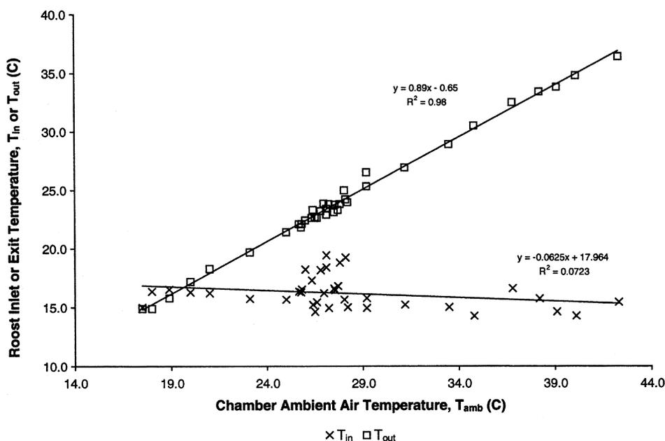
Figure 2. Roost calibration curve used to estimate roost exit temperature without birds ( $T_{out}$ ).
