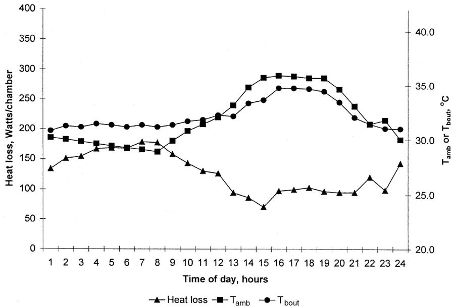
Figure 4. Plot of day 40 average heat loss through birds' feet to the cool roost system and corresponding ambient air ( $T_{amb}$ ) and cool roost water exit temperature ( $T_{bout}$ ) in flock 2.
