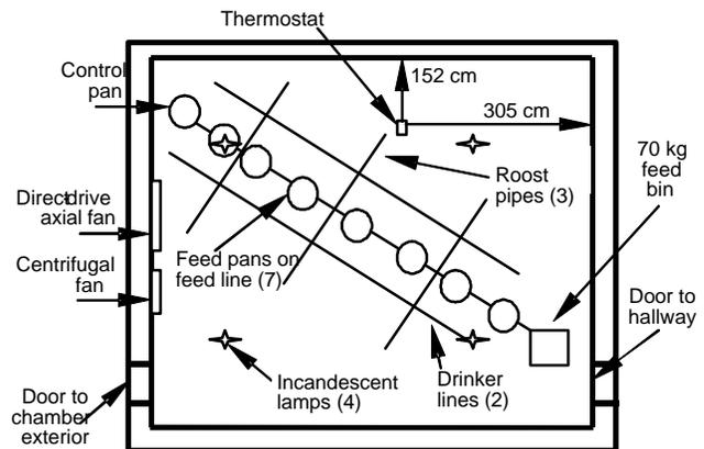
Figure 1. Chamber layout showing lighting, ventilation, roost, feeding, and watering systems in a chamber used in the studies. Light bulbs were located 1.5 m from the nearest wall.
