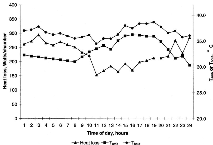
Figure 3. Plot of day 39 average heat lost through birds' feet to the cool roost system and corresponding ambient air temperature ( $T_{amb}$ ) and cool roost water exit temperature ( $T_{bout}$ ) in flock 2.
